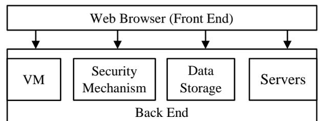
Fig.1. Cloud computing architecture
