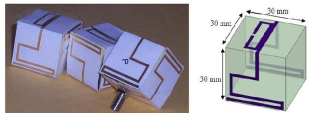
Fig.4. A view of the antenna used in the proposed protocol [18]
