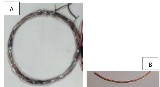
Fig.4. The developed coil photos (a) Close view of the designed coil (b) Close view of the copper wire used in the coil
