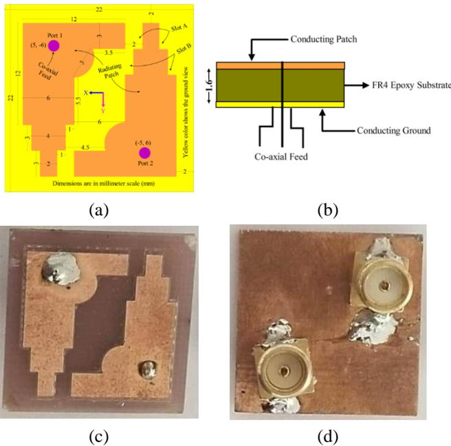
Fig.1(a-b). Upper-view (orange), lower-view (yellow), middle-view (green) and (c) fabricated upper-view, (d) fabricated lower-view of the proposed antenna ( $A_4$ )
