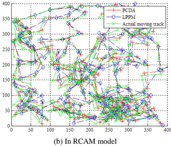
Fig.6. Comparison between actual track of the target and predicted track of it
