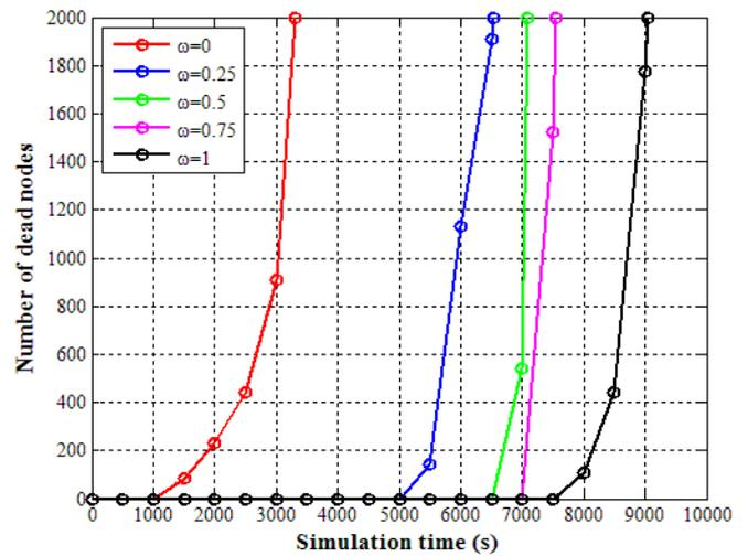
Fig.2. Number of dead sensors versus simulation time in different  $w$
