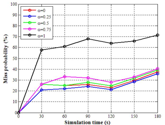
Fig.3. Missing probability versus simulation time in different  $w$
