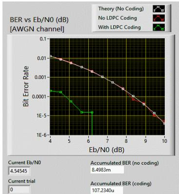
Fig.10. BER vs.  $E_b/N_o$  with LDPC in PSK modulation
