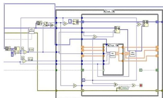
Fig.3. Labview implementation of LDPC encoder
