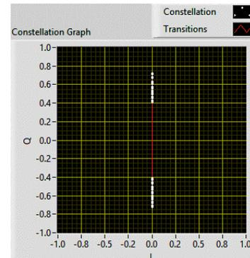
Fig.8. PSK Modulation Constellation Graph
