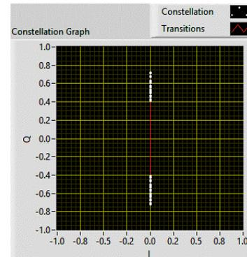
Fig.8. PSK Modulation Constellation Graph
