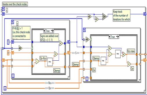
Fig.4. Labview implementation of the LDPC decoder
