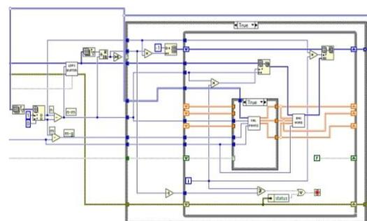
Fig.3. Labview implementation of LDPC encoder
