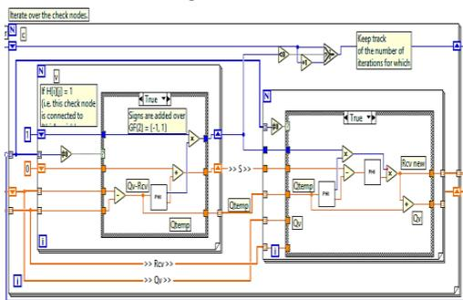
Fig.4. Labview implementation of the LDPC decoder
