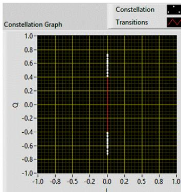
Fig.11. PSK modulation constellation graph (with LDPC)
