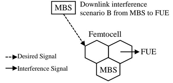
Fig.1. Downlink Cross-tier interference scenario B in femtocell networks
