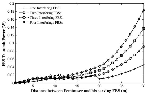
Fig.6. Neuro-controller adjusted FBS transmit power for the case of increasing quantity of interfering FBSs
