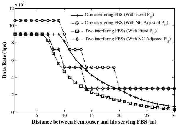
Fig.4. Achieved data rate of femtocell user with one and two numbers of interfering FBSs
