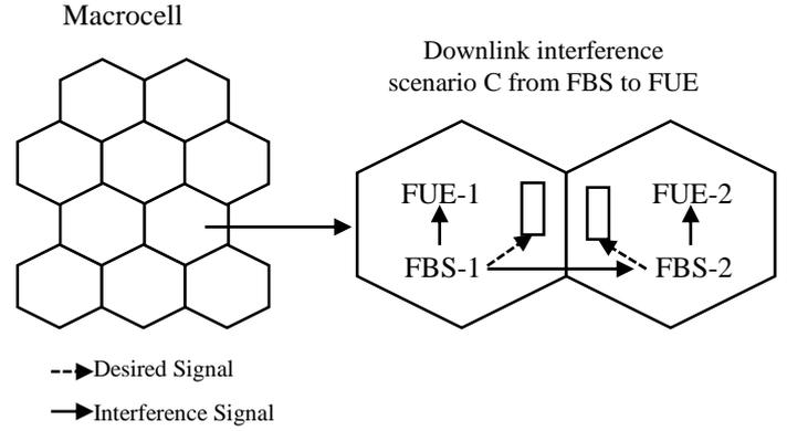
Fig.2. Downlink co-tier interference scenario C in femtocell networks
