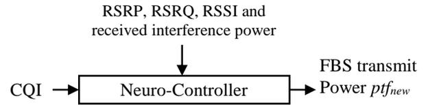
Fig.3. Block Diagram for Intelligent FBS Transmit Power Control
