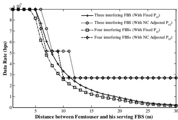
Fig.5. Achieved data rate of femtocell user with three and four numbers of interfering FBSs
