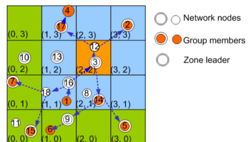
Fig.1. Example of Zone Structure
