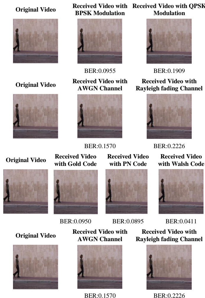
Fig.6. Colour video received respectively with various codes, channels, modulations and with conventional rake receiver and CBKFR receiver at SNR = 20dB
