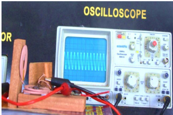
Fig.18. Arrangement of WPT system ( D = 2\text{cm} , Input Voltage: 5V)
