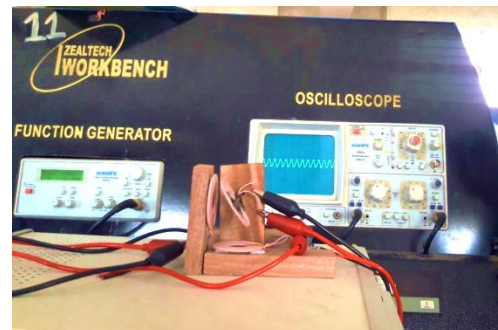
Fig.17. Arrangement of WPT ( D = 1\text{cm} , Input Voltage: 5V)
