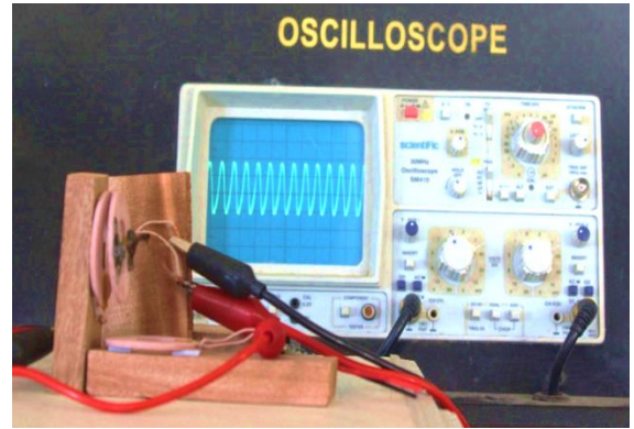
Fig.16. Arrangement of WPT D = 0\text{cm}
