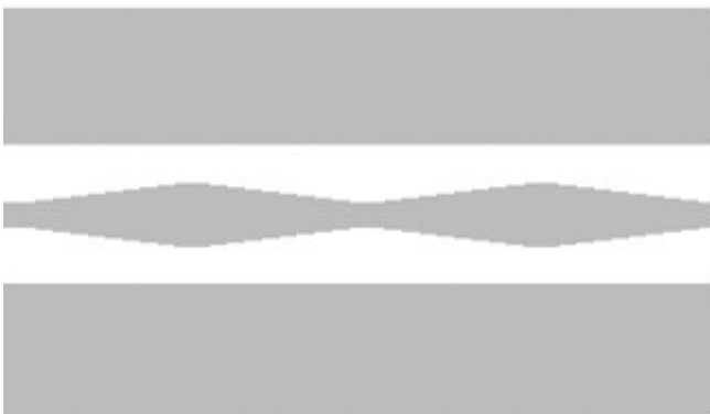
Fig.6. A Bow-Tie tapered CPW having 2 sections
