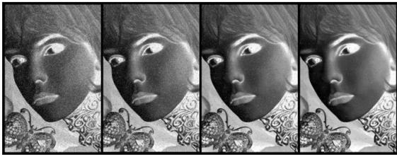
Fig.11. Image transmission using TCOFDM (rate  $\frac{1}{2}$ ) with soft decoded QPSK modulation at  $E_b/N_0=0$  dB for iterations 1, 2, 5, and 9 respectively
