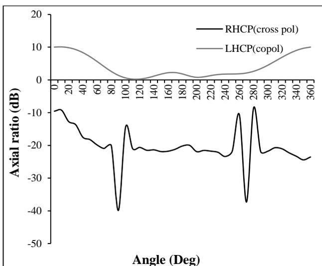
Fig.11. simulated results of co polarization (LHCP) and cross polarization (RHCP) of proposed antenna for CP case at 5.19MHz
