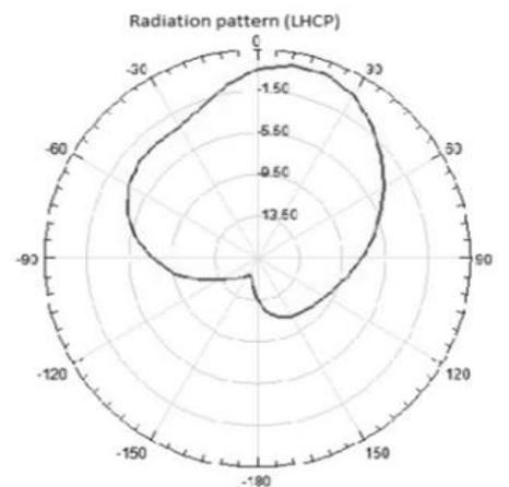
Fig.9(c). Radiation pattern of the proposed antenna for LHCP case
