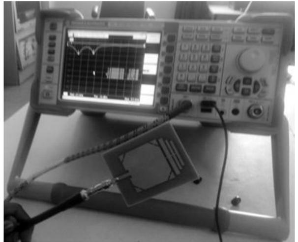
Fig.2. Photo copy of fabricated antenna with practical setup
