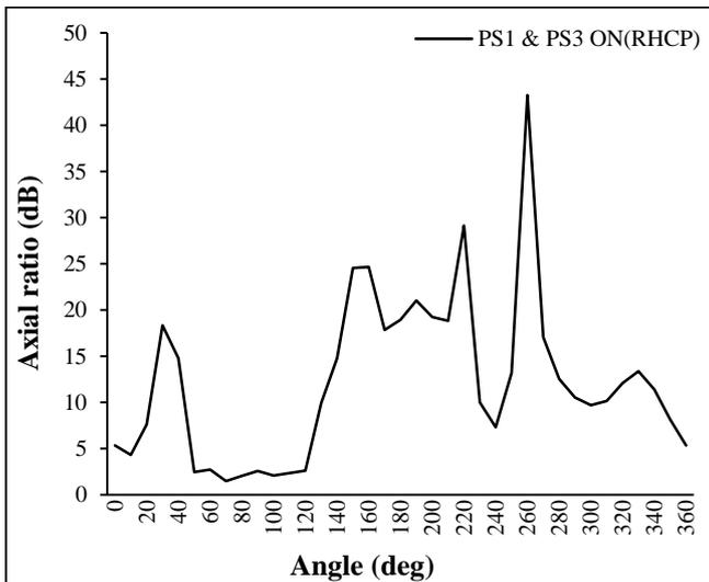
Fig.8. Simulated axial ratio characteristics of the for RHCP
