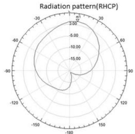
Fig.9(b). Radiation pattern of the proposed antenna for RHCP case
