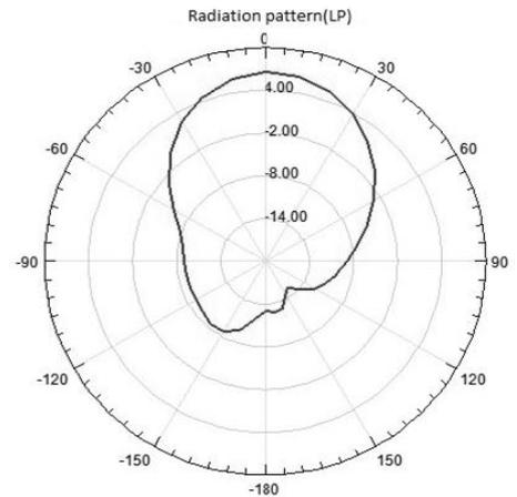
Fig.9(a). Radiation pattern of the proposed antenna for LP case
