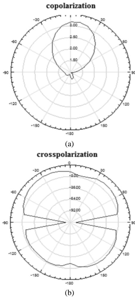
Fig.10. Simulated results of (a). Copolarization and (b). Cross polarization of proposed antenna for LP case at 5.19MHz
