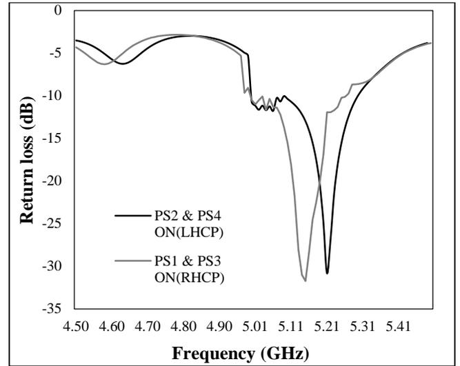
Fig.5. Simulated return loss characteristics of the antenna for LHCP & RHCP
