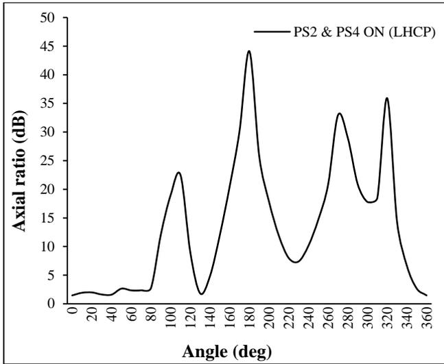
Fig.7. Simulated axial ratio characteristics of the antenna for LHCP
