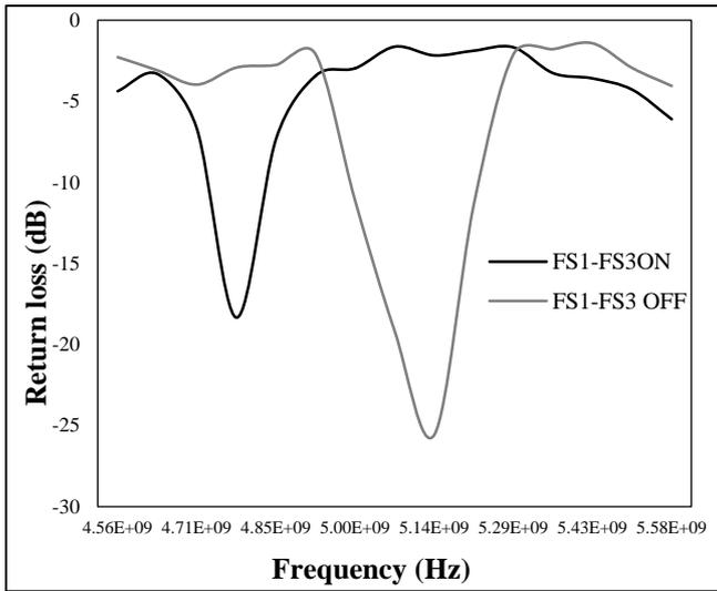
Fig.4. Measured return loss characteristics of the antenna
