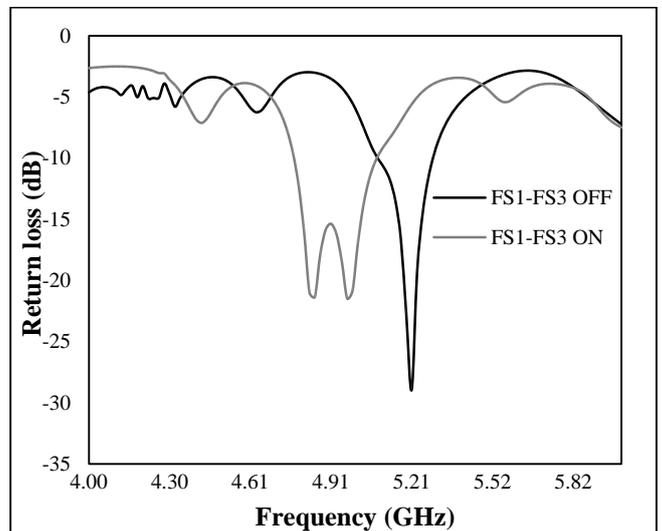
Fig.3. Simulated return loss characteristics of the antenna
