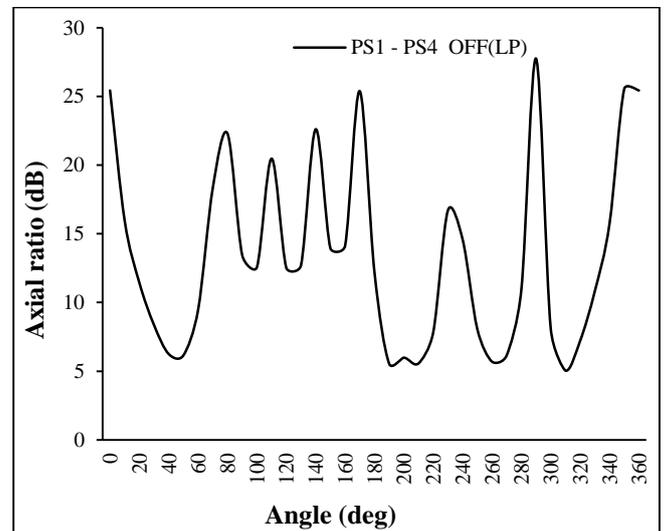
Fig.6. Simulated axial ratio characteristics of the antenna for LP
