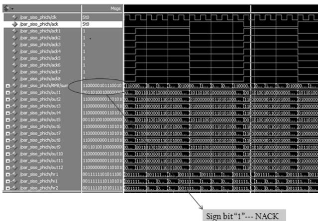
Fig.15. Simulation Wave for PHICH Receiver
