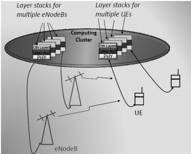
Fig.3. Flow-diagram for the centralized processing
