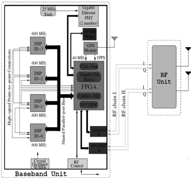
Fig.5. Block diagram of Baseband unit
