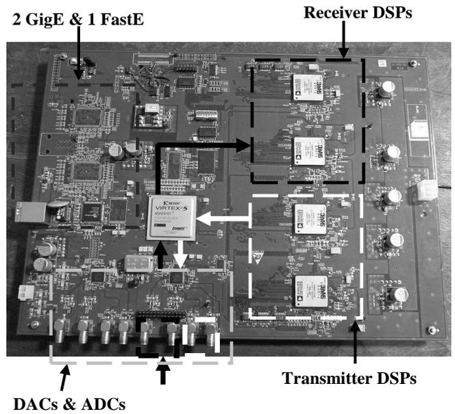
Fig.6. Picture of the prototype Baseband section
