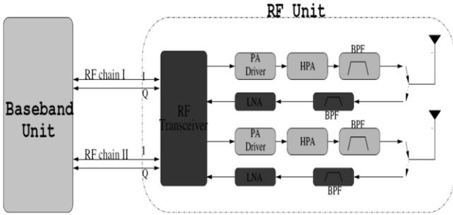
Fig.2. Block-diagram of the Baseband and RF unit
