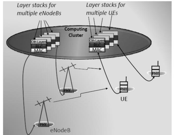
Fig.4. Flow-diagram for the distributed processing
