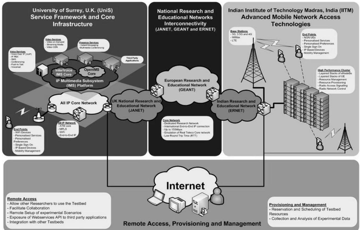
Fig.7. High level integrated view of Access, Core and Service delivery testbed
