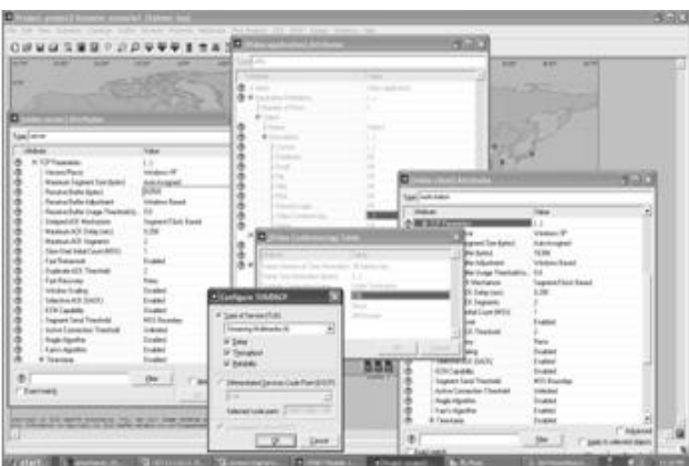
Fig.6. Configuring the Simulation Environment for Video Transmission using TCP with ToS 156
