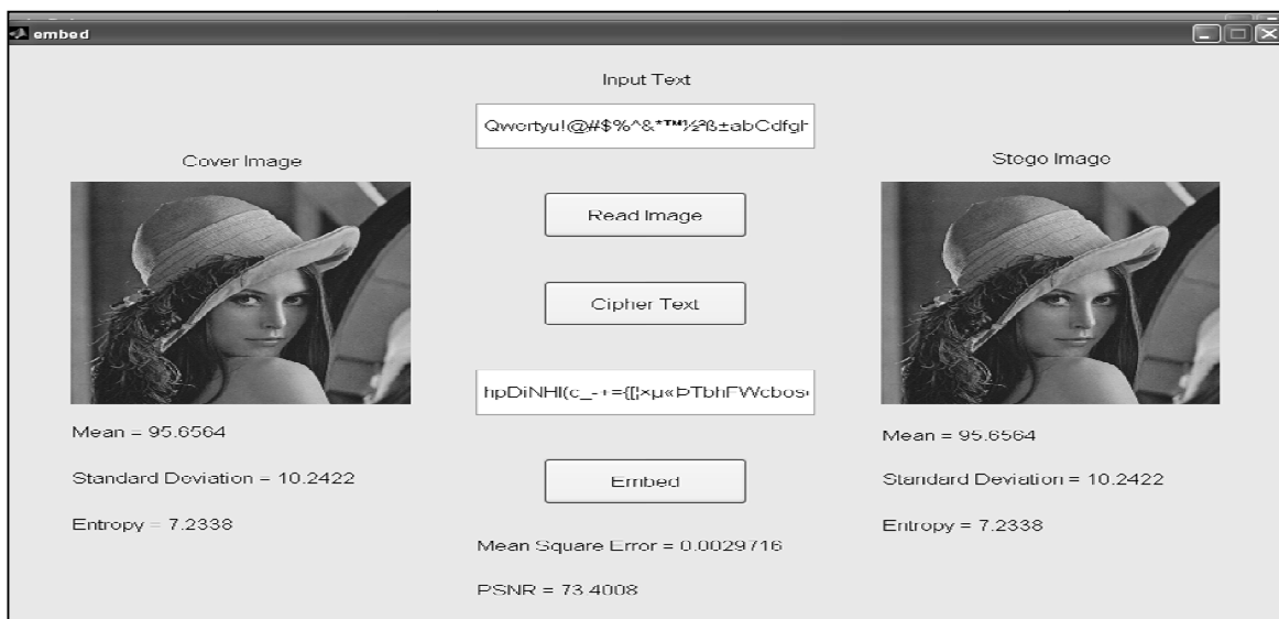
Fig.7. Graphical user interface of Three LSB Steganography for 300 characters
